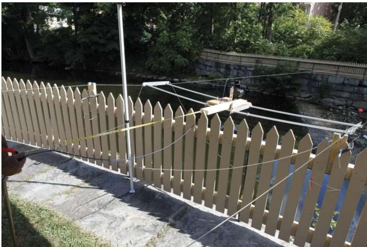
Hand-built apparatus for maneuvering a medium-format digital camera over canal at Francis Gate, Lowell, MA. Courtesy of Miles Coolidge.
